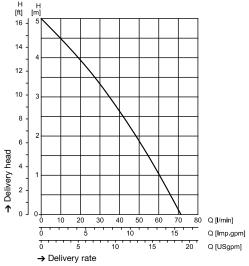
Data are for liquids with a viscosity of 1 mm<sup>2</sup>/s and a density of 1 kg/dm<sup>3</sup>
